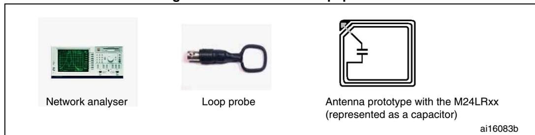
This equipment setup will directly display the system's resonant frequency.
