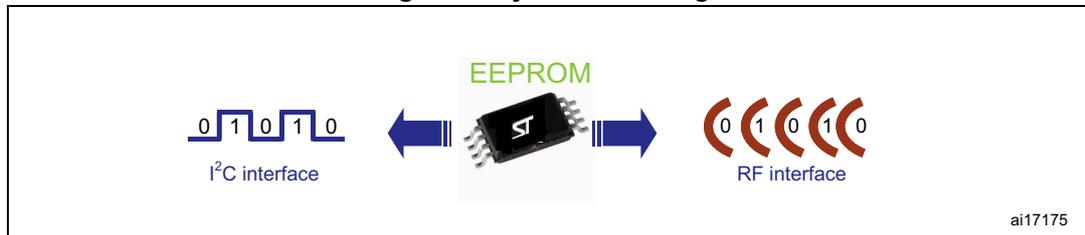
Dynamic NFC tag can be used in many applications, with the requirement that the processor features an I<sup>2</sup>C interface.
