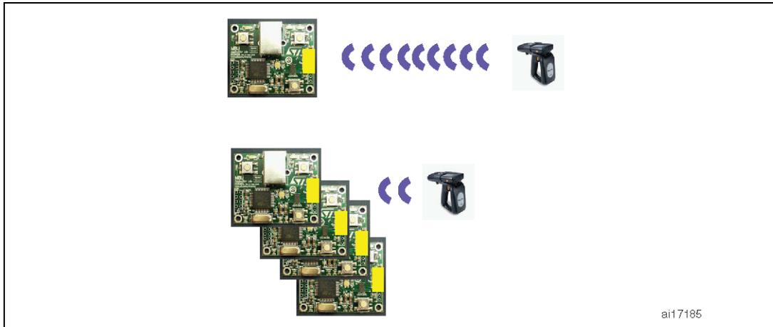
The vicinity of another dynamic NFC tag board may change the inductance dynamics. The boards may couple with each other, leading to a resultant antenna resonant frequency different from the individual one.
