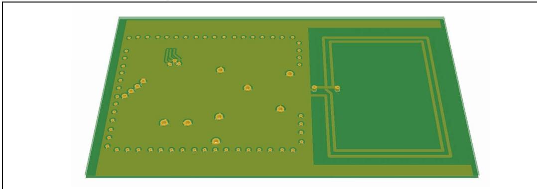
It is recommended to allocate a dedicated area of the PCB layout to the antenna only, with no surrounding ground layer, as shown in [Figure 13](#).
