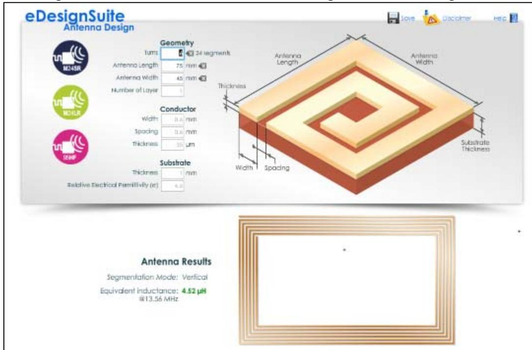
Figure 11 shows an example of antenna computation, the following parameters have to be defined:
