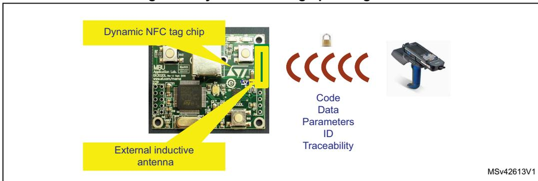
The design of an antenna for dynamic NFC tag is based on the placement of a loop on the application PCB. Its impedance matches the device internal tuning capacitance value ( $C_{\text{tuning}}$ ) to create a circuit resonating at 13.56 MHz. The basic equation of the tuning frequency is:
