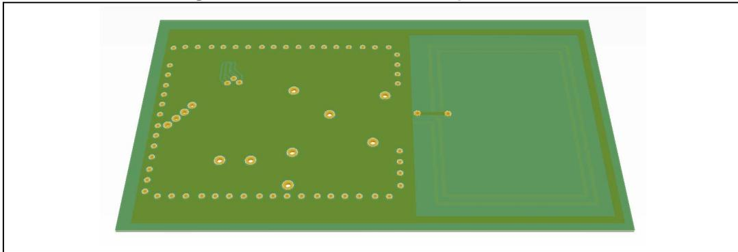
Figure 17 shows an acceptable implementation, here the antenna and the ground plane do not overlap.
