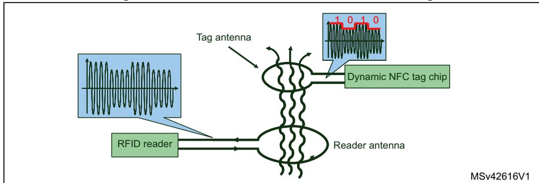
At the end of the request, the reader keeps the magnetic field non modulated to power the tag, and allows it to generate an answer. To send its response back to the reader, the dynamic NFC tag chip backscatters the data to the reader by internally modulating its input impedance. Tag chip input impedance variation modulates the signal across the reader antenna due to the mutual coupling between reader and tag antennas. The reader demodulates this signal and decodes the tag answer.
