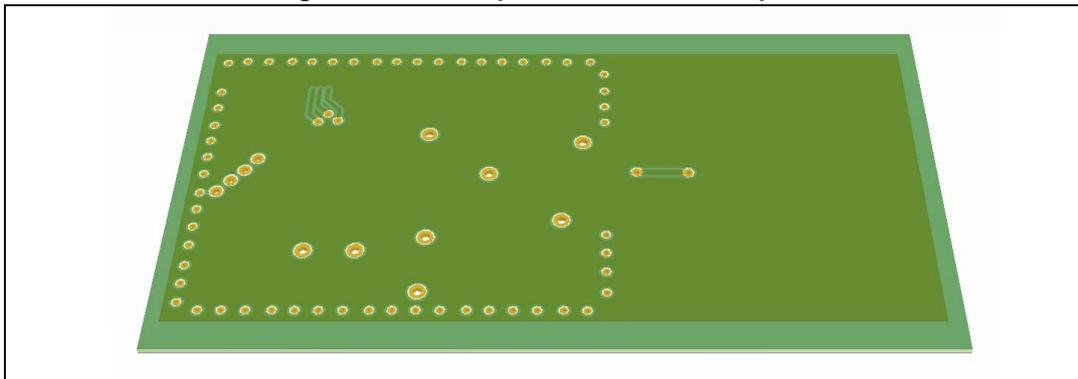
Figure 16 shows an example of a not recommended implementation. The electromagnetic flux is greatly attenuated by the short-circuited loop surrounding the dynamic NFC tag antenna.
