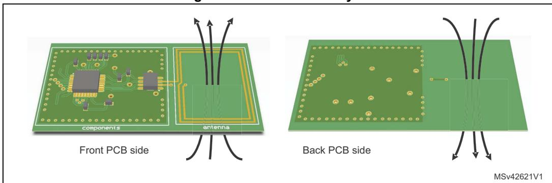
The energy transfer and the communication between the reader and the dynamic NFC tag are suitable because no copper planes overlap the antenna.
