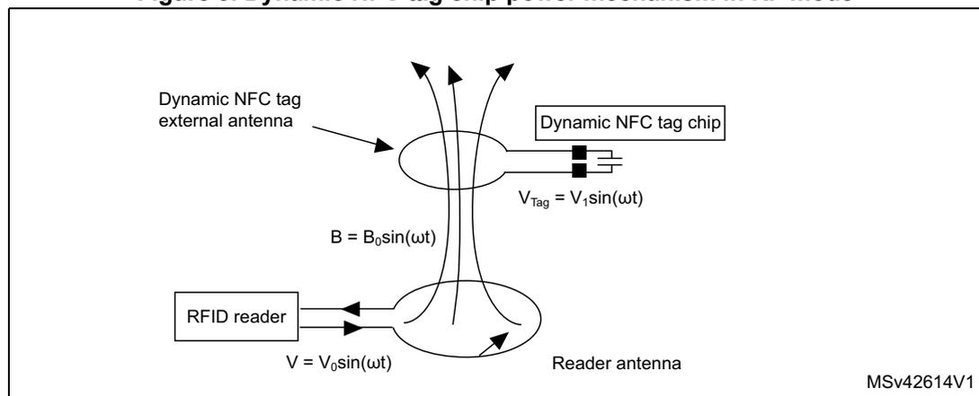
When the dynamic NFC tag is placed in the RFID reader’s electromagnetic field, the amount of energy powering the device is directly related to the orientation of the dynamic NFC tag antenna and to the RFID reader antenna. Indeed, this energy depends on how the electromagnetic field lines generated by the reader flow through the dynamic NFC tag antenna (see [Figure 4](#)).
